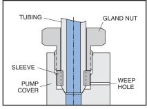
Typical Coned and Threaded port connection
